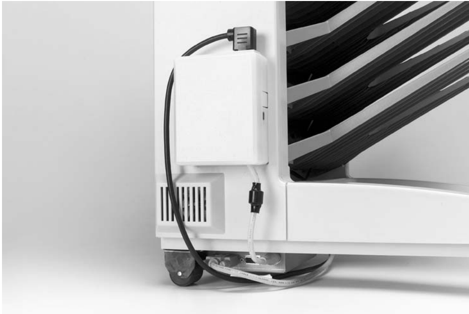
Figure 7-24 8-bin Mailbox Power Supply Test Mode Switch
